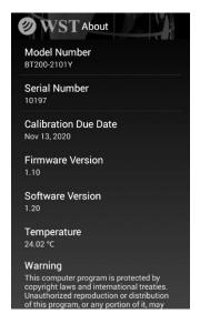
The *About* screen provides information relating to the BT200. The information provided includes the Model Number, Serial Number, Calibration Due Date, Firmware Version, Software Version, and internal temperature of the BT200.
