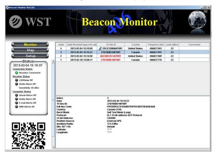
Connect the FBM200 receiver to a USB port on the computer using the supplied USB cable. This connection is both the power supply and the communication link to the receiver. When the FBM200 receiver is located, the Connection Status in the Status section will show *Connected*.
